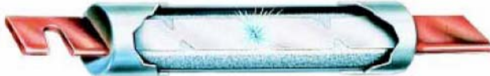
Figure 2. Under sustained overload, a section of the link melts and an arc is established.
