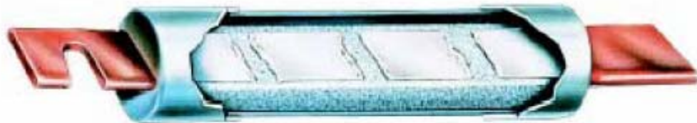
Figure 5. The “open” single-element fuse after opening a shorted circuit.
