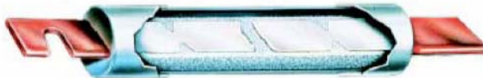
Figure 3. The “open” single-element fuse after opening a circuit overload.
