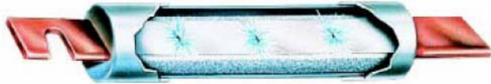
Figure 4. When subjected to a short-circuit current, several sections of the fuse link melt almost instantly.
