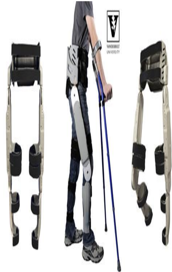
Figure 2. Exoskeletal components of hybrid neuroprosthesis. Knee joints are instrumented with solenoid controlled wrap-spring clutches that provide support during stance and unlock for swing. Hip mechanism, depicted schematically with accumulator and valves, includes hydraulic rotary actuators attached to hips and controlled by variable constraint hip mechanism. Postural controller uses information from force-sensitive resistors, potentiometers, optical switches, and pressure sensors to regulate hip and knee mechanisms to maintain exoskeletal stability against collapse and to provide freedom to move legs with functional electrical stimulation.
