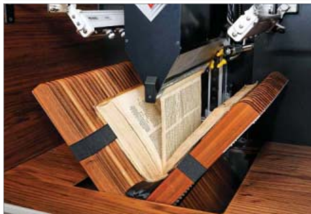
A DELICATE TASK: A pair of extra-gentle digitizing robots scan books at the Bavarian State Library. PHOTOS: TREVENTUS MECHATRONICS
