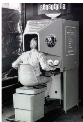
NOW AND THEN: The Oculus Rift [top] is the latest in a long line of attempts to make virtual reality commonplace, some of which include Morton Heilig's creation in 1962 of the electromechanical Sensorama [bottom left]; NASA's work in the 1980s on a system that allowed wearers to interact with scenes using data gloves [bottom middle]; and Nintendo's 1995 Virtual Boy [bottom right], which was a spectacular flop.
