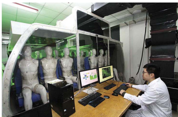
THE BIG DEBUT: Comac celebrated the first C919 to roll out of the factory in early November of 2015 [top]. A mock-up of the new plane's passenger cabin [bottom] was used to develop the ventilation system.
