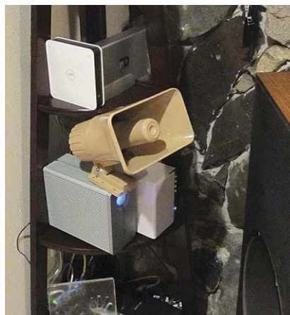
HOME-BREW HOUSE GUARD: A microphone connected to a Wi-Fi-enabled Arduino Uno listens for the Scout's alarms. A wireless switch turns on the siren.
