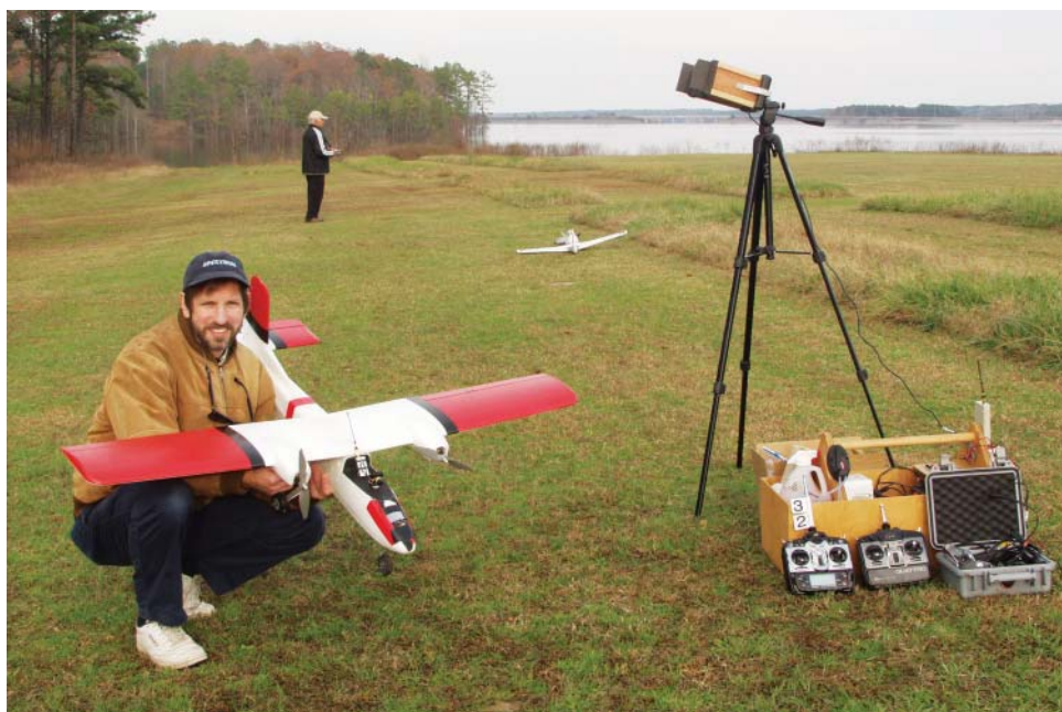
MICRO DRONE: Adding a video camera and radio downlink to a radio-controlled model airplane has become easy. PHOTO: DAVID SCHNEIDER
