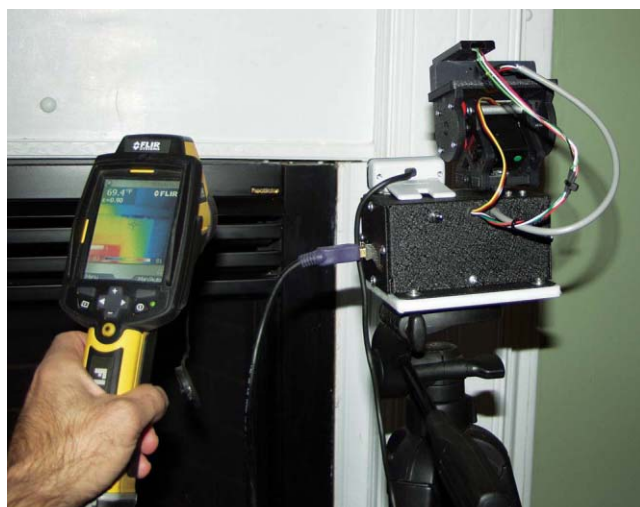
FACE-OFF: A commercial thermal imager [left] produces higher-resolution images and works much faster, but the tripod-mounted Cheap Thermocam [right] does basically the same job—and on a budget. PHOTO: DAVID SCHNEIDER
