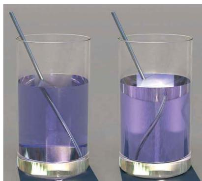
**A NEGATIVE BENT:** Artificial materials can be made to have a negative index of refraction, a light-bending property not seen in nature. The interface of air and water—two substances with positive indices—creates a small kink in the appearance of a straw [left]. If the liquid had a negative index of refraction, the straw would appear to bend in the opposite direction [right].
