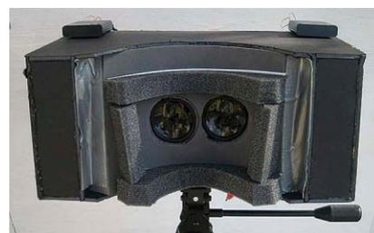
**AIR SHOW:** I mounted two video cameras on my plane to provide stereoscopic vision, each with its own transmitter [top]. Images were displayed on two screens in the headset [left] and then brought via mirrors to the eyepieces [above].
