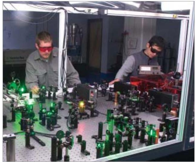
**LIGHTING THE WAY:** A new tabletop extreme ultraviolet laser.
