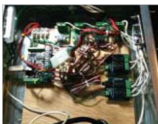
SMART STRIP: Lay in wires for the buttons and LEDs first [upper left]. Mount an I/O board with sensors and relays [upper right] on a piece of wood—and make sure your enclosure is big enough [lower left]. If you wired correctly, an LED will light up when a plug is live [lower right]. PHOTOS: JAMES TURNER
