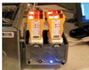
SMART STRIP: Lay in wires for the buttons and LEDs first [upper left]. Mount an I/O board with sensors and relays [upper right] on a piece of wood—and make sure your enclosure is big enough [lower left]. If you wired correctly, an LED will light up when a plug is live [lower right]. PHOTOS: JAMES TURNER
