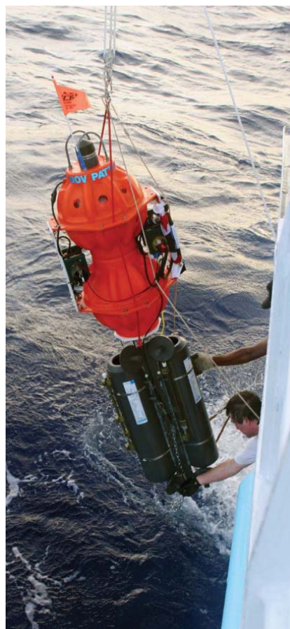
LANDER AWAY: During the July expedition to the Mariana Trench, marine engineer Kevin Hardy [top] prepares the seafloor lander's sample tubes. Researchers hope that water samples from more than 10 000 meters down will contain strange new life-forms. Once the lander begins its plunge [bottom], it takes 3 hours to reach the seafloor.
