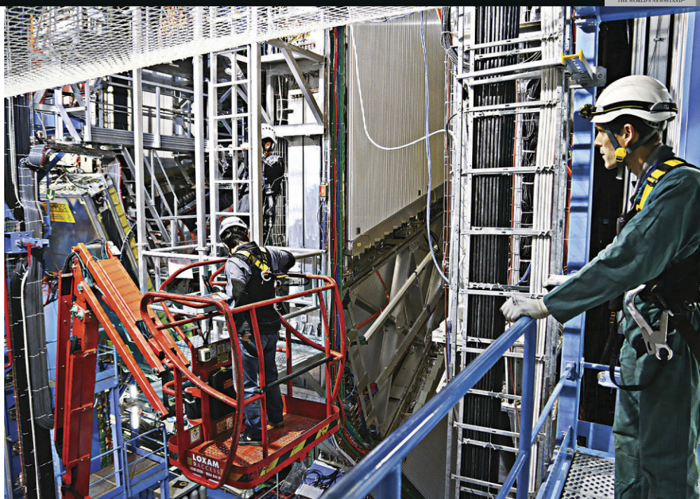
BACK WHERE IT BELONGS: A muon chamber is slotted into place in preparation for the restart of the Large Hadron Collider.
