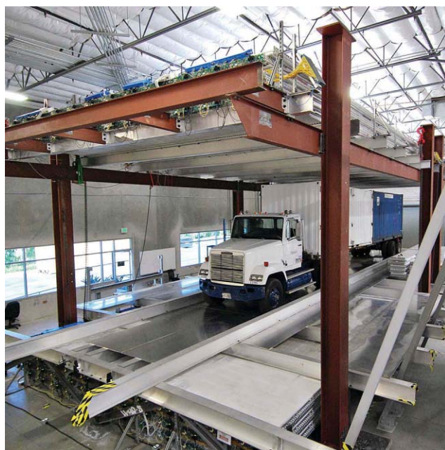
PROTECTING PORTS: At its R&D center, Decision Sciences demonstrates how its muon-scattering imaging system can be used to screen for smuggled nuclear materials at borders.
