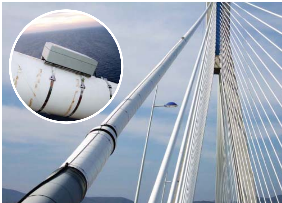
HIGH IQ: Accelerometers, tiltmeters, and strain gauges send their signals to remote engineers. PHOTOS: ADVITAM
