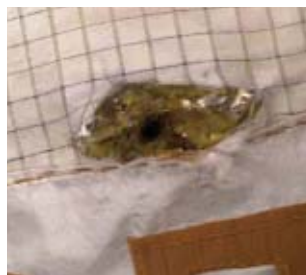
METEOROID DAMAGE: Pictured are the results of impacts on the Atlantis space shuttle payload bay door radiator, an insulation blanket on a module of the International Space Station, and the Hubble Space Telescope solar array.
