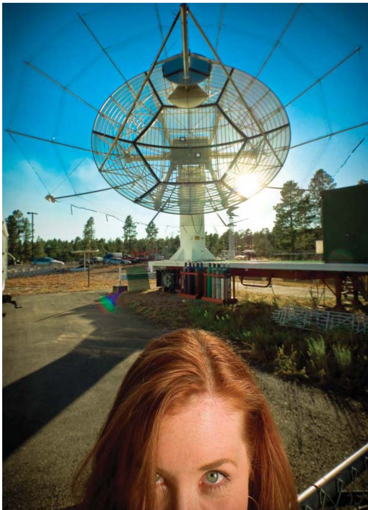
STAR TRACK: The author with the Los Alamos Portable Pulsar, which beams VHF signals that satellites can detect. PHOTO: CHIP SIMONS
