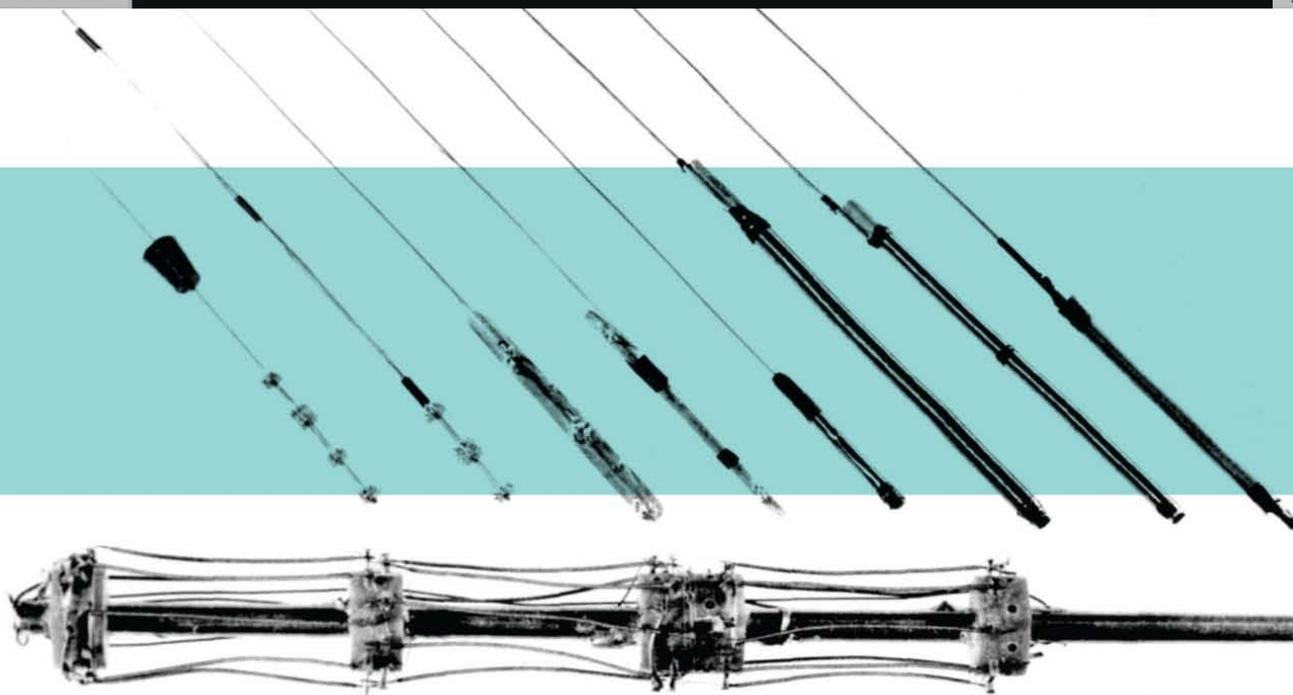
**MADE BY HAND:** Buck [right] fashioned many prototypes, including a multivibrator circuit [close-up, above], the schematic for which reveals 19 individual cryotrons [below]. With this technology, he anticipated, engineers could construct a bread-box-size computer as powerful as MIT's Whirlwind [far right].
