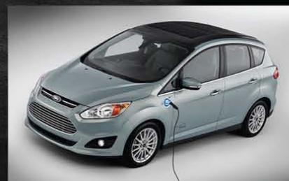
**PRICE:** Not for public sale **POWER TRAIN:** 2.0-L four-cylinder with electric motor; 140 kW (188 hp) total power **OVERALL FUEL ECONOMY (EST.):** 5.5 L/100 km (43 mpg) on gasoline; energy equivalent of 2.35 L/100 km (100 mpg) on battery
