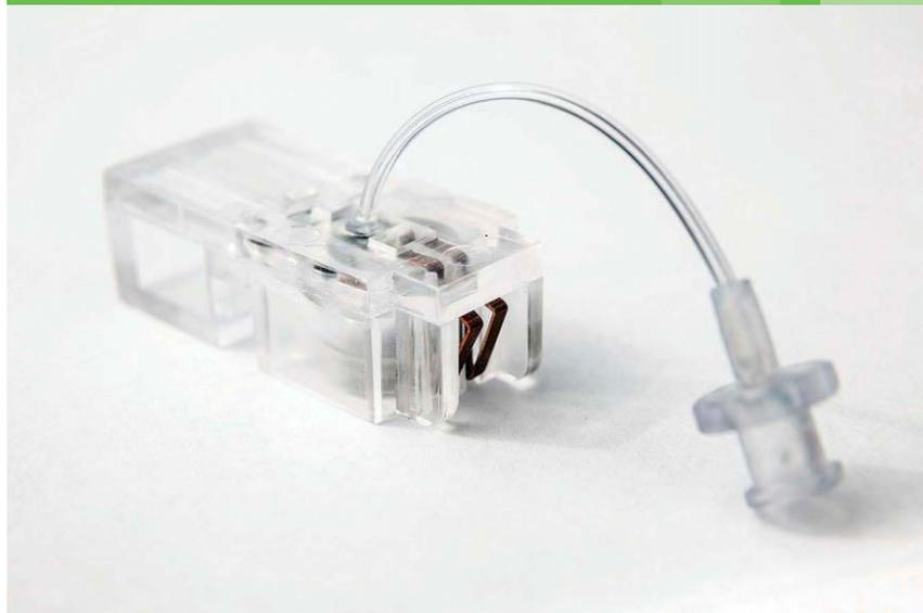
**SUPERBUG SUPERSLEUTH:** F Cubed's chip uses an electric field to tease out the presence of a MRSA bacterium's DNA.
