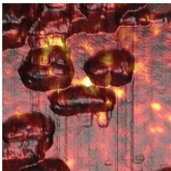
**A CRUCIAL COATING:** Metal nanocages [brown] deposited on the surface of a fiber probe induce hot spots of electromagnetic energy [yellow] in this composite image. This layer increases the sensitivity of a lab on fiber by as many as four orders of magnitude.
