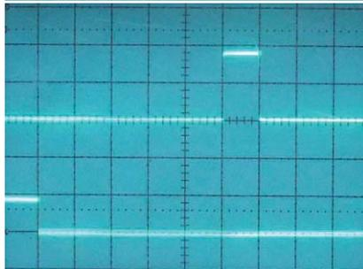
**JOSEPH ALLEN'S INSPIRATION** was a 1960s calculator that used delay-line memory [top]. His acoustic delay line uses a collection of amplifier and logic chips [second from top]. An oscilloscope displays the bits 0011 flowing through the delay line [second from bottom] and the result of inverting a bit [bottom].
