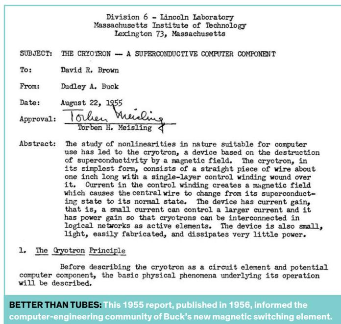
Through the rest of 1955, Buck's personal cryotron research at MIT focused on creating miniature cryotrons, and even integrated cryotron arrays, using evaporated thin films. Instead of winding small wires about one another, he wanted to evaporate metal through a mask, like a stencil, onto a substrate to create a patterned thin film of superconducting material. Atop this film, he would evaporate the control wiring through another mask. He would thus be able to print cryotrons, arrays of them.
