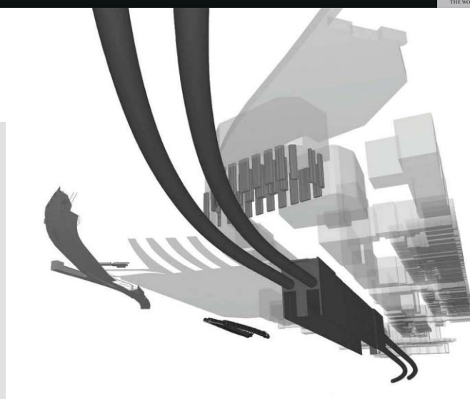
VIRTUAL MEETS REALITY: A point-cloud survey of Paddington station [above] uses laser scanning to ensure that construction conforms to building plans.
