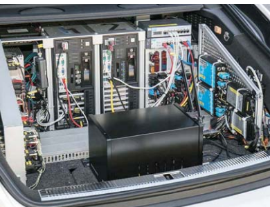
BRAIN IN A BOOT: The Audi RS7's computing hardware fills the trunk space.
