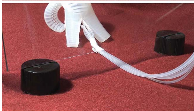
ROBOT LIMBO: A soft robot at Harvard University takes advantage of its rubbery nature to maneuver under an obstacle.
