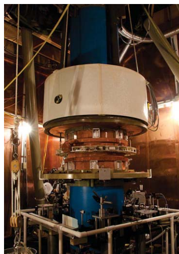
PURSuing PLANCK: The NIST watt-balance [left] and the NRC watt-balance [right] experiments are two leading efforts to measure Planck's constant.
