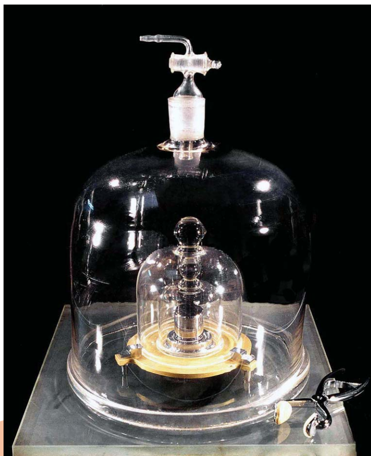
CYLINDERS AND SPHERES: The International Prototype of the Kilogram [left] is kept in a vault near Paris. One effort to redefine the kilogram measures ultrapristine silicon spheres. Two spheres are cut from a single crystal [top left] and polished [top right]; the spheres are then weighed with high precision against other objects in comparators like this one [bottom].
