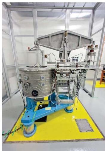
PURSuing PLANCK: The NIST watt-balance [left] and the NRC watt-balance [right] experiments are two leading efforts to measure Planck's constant.
