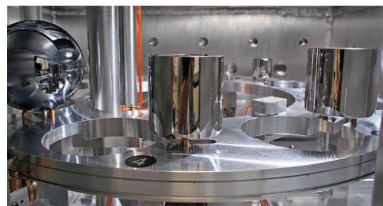
CYLINDERS AND SPHERES: The International Prototype of the Kilogram [left] is kept in a vault near Paris. One effort to redefine the kilogram measures ultrapristine silicon spheres. Two spheres are cut from a single crystal [top left] and polished [top right]; the spheres are then weighed with high precision against other objects in comparators like this one [bottom].
