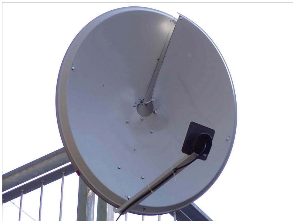
SLIGHT TWIST: Bending a dish antenna allowed researchers to project twisted radio waves.
