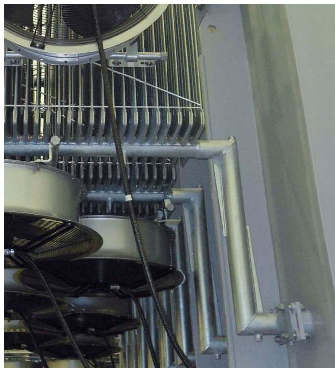
FIGURE 5: Top: The thermo-fluid dynamics simulation of the new design. Bottom: New collecting pipes design. In the new design, the pipes have been removed from their previous position circling exterior of the reactor. Instead, the pipes travel directly from the cooling fan and into the reactor itself.
