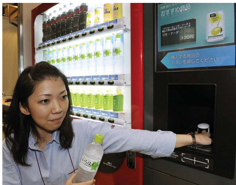
PAYMENT BY FINGER: At a technology expo, a Hitachi employee shows off a prototype of a biometric-based vending machine. PHOTO: YOSHIKAZU TSUNO/AFP/GETTY IMAGES
