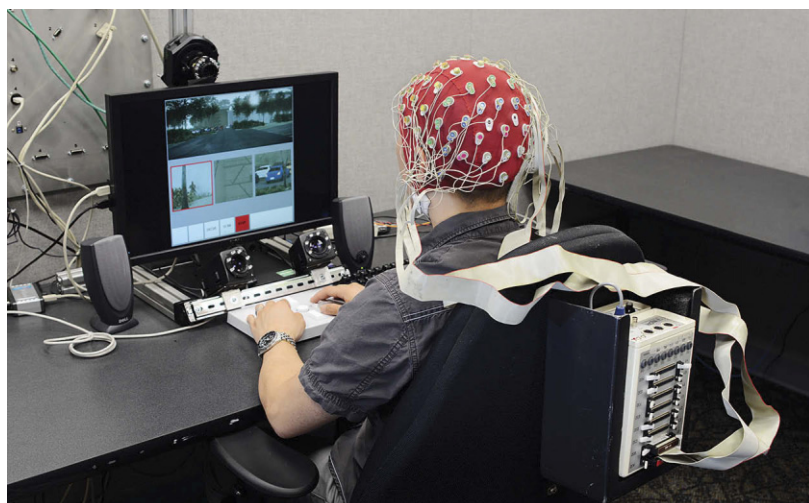
MIND-READING MACHINE: A volunteer tests a brain-computer interface being developed at the U.S. Army Research Laboratory. The system can identify when a user spots a potential threat, such as a person with a gun, simply by observing brain activity.
