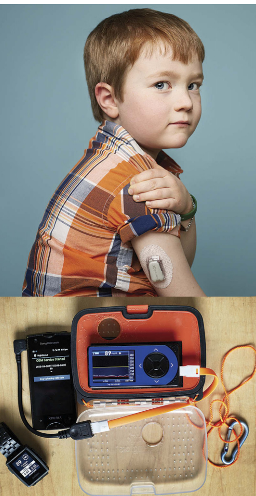
PEACE OF MIND: Evan wears a blood-sugar sensor and transmitter [top]. A box contains the receiver and a smartphone, and a Pebble watch lets his parents monitor his sugar levels.
