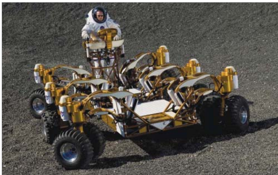
MOVE OVER, BEN HUR: Chariot, a lunar truck prototype designed at the Johnson Space Center, has six double wheels that can be steered independently in any direction and a tanklike turret that rotates 360 degrees.
