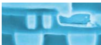
A scanning electron microscopy image of a copper line interconnect where a void has developed due to vacancy accumulation.
