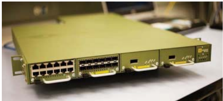
FLOW CONTROL: The Anagran FR-1000 can be plugged into existing networks and can manage up to 4 million simultaneous flows.
