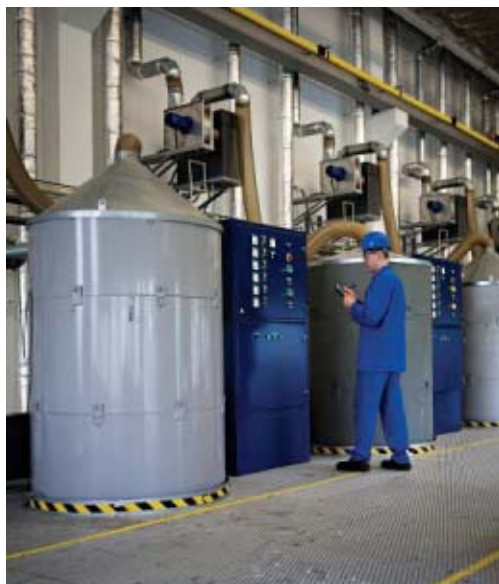
AMMONO'S AUTOCLAVES: In a single run, they now produce over 70 2-inch crystals of gallium nitride.
