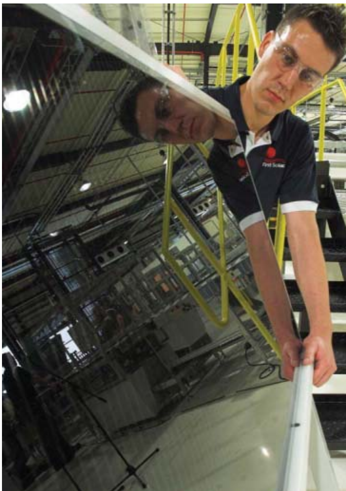
A RARE LOOK inside a First Solar plant—here, in Frankfurt/Oder, eastern Germany—gives away none of the company's secrets, which involve manufacturing very large panels. The cell structure itself is known [see diagram below]; as in all thin-film designs, the active layers are built on an inert glass wafer.
