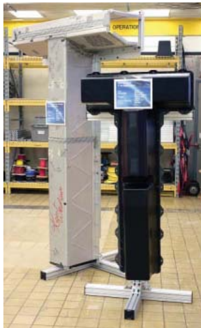
NEXT GENERATION: The battery pack that will be used for the Chevrolet Volt [right] poses next to its older sibling, the original EV1 battery pack. PHOTO: JOHN F. MARTIN/GENERAL MOTORS
