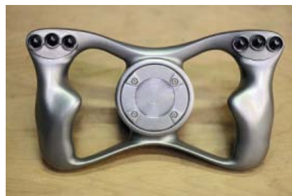
HAND IN GLOVE: The steering wheel was formed of hollow titanium to fit Andy Green’s hands. It is light, yet tough enough to take wild handling should the planned straight-arrow course go awry.
