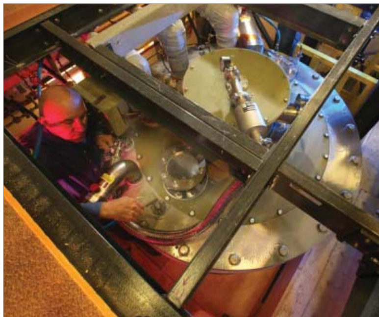
MAGNETIC MOMENT: Engineers are readying a supercooled, record-setting 100-tesla magnet at Los Alamos National Laboratory. The magnet will have to withstand forces equivalent to 200 sticks of dynamite. PHOTO: LEROY N. SANCHEZ/LOS ALAMOS NATIONAL LABORATORY
