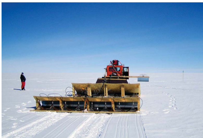
ARRAY OPTIONS: The multiple antennas required by the new system may be either mounted under an aircraft [top] or pulled on a sled by a tracked vehicle [bottom].
