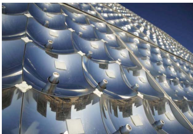
HIGH MAGNIFICATION: Focusing sunlight on photovoltaic cells not only reduces the chip costs of the system but also boosts efficiency. That's because the more intense the light gets, the higher the voltage and the output power become. PHOTO: SOLFOCUS
