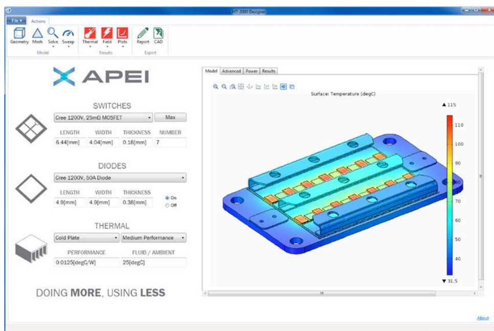
A COMSOL® software simulation application created at APEI for predicting the performance of different power module designs.
