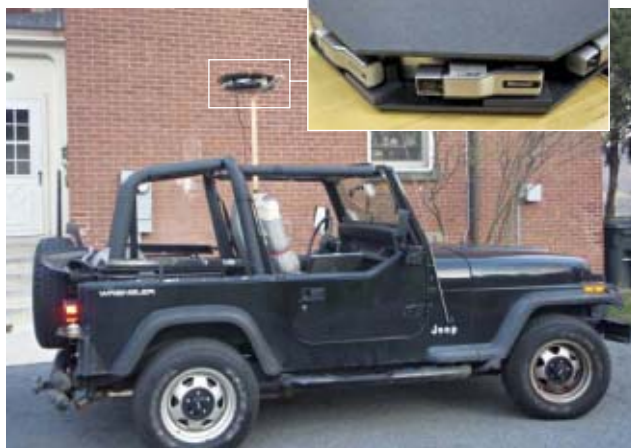
JEEP CAM: Mounted on a moving vehicle, the camera array [detail] can capture images of streets and their surroundings—just as Google does to produce its Street View panoramas.
