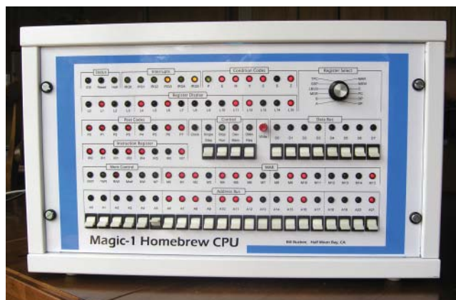
FLASHBACK: The front panel of Bill Buzbee's handcrafted Web server [left] evokes the late 1960s or early '70s. Residing within it are some two hundred 74-series ICs, painstakingly wire-wrapped together [right].
