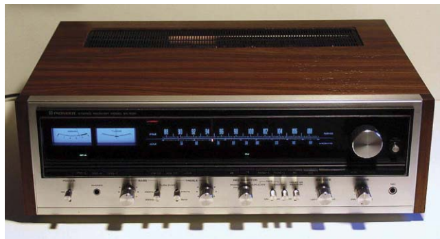
SEVENTIES SOUND: This Pioneer SX-838 receiver, manufactured circa 1975, can output 50 watts per stereo channel. PHOTO: TIM WHYTE
