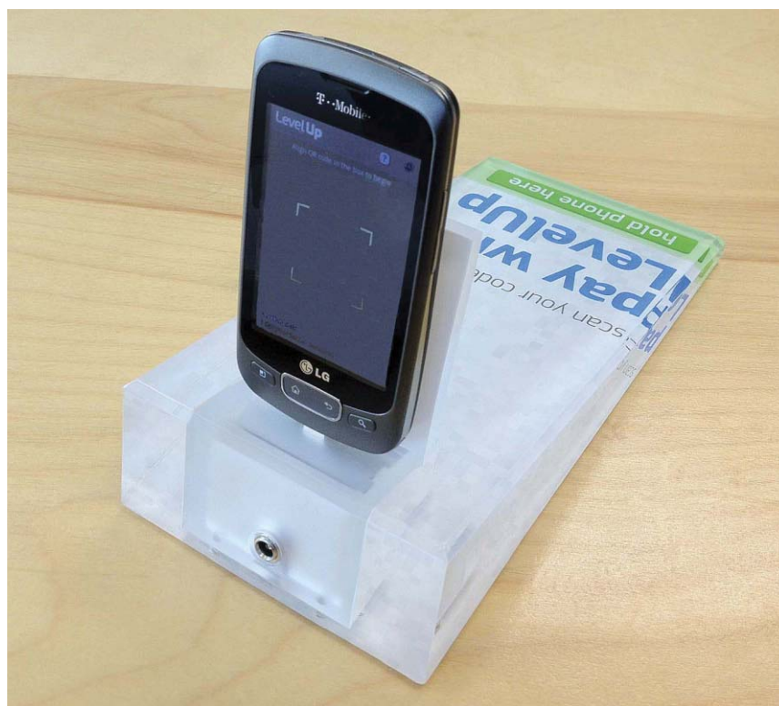
PAY HERE: An app on a customer's smartphone generates onscreen payment bar codes and records progress toward a reward [above]. LevelUp's reader [left] is based on a 3G smartphone and uses its camera to record the bar codes. PHOTO: STEPHEN CASS; SCREEN SHOT: LEVELUP
