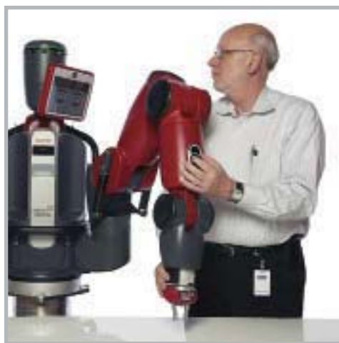
PROGRAM ME, PLEASE: Product manager Mike Bugda demonstrates how to program Baxter to perform a new task. He simply holds the arm by the cuff and moves it to the desired location. He tells the robot what to do using a knob and buttons.
