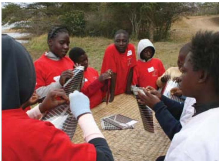
FIELD TEST: Students in Zambia test early polymer photovoltaic-powered lights developed in Denmark. PHOTO: FREDERIK KREBS
