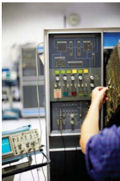
BACK TO THE FUTURE: An IBM 1401 system [left] filled a room. Its equivalent now fits in your hand. The CPU operator's panel [below] shows data lines linking registers, switches, and memory.
