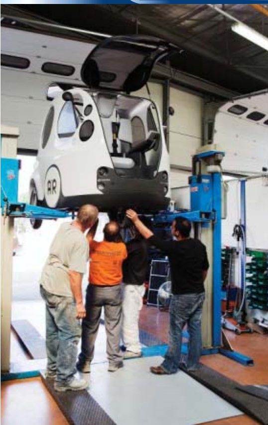
POD SQUAD: Workers at Motor Development International are busy readying AirPod prototypes at the company's fabrication facility near Nice, France. Viewed from underneath its curvaceous shell [left], the AirPod reveals an aluminum frame, which encloses a composite tank holding air compressed to 350 bars [middle]. A steering wheel would be impractical, because the driver's door is located at the front of the vehicle. The solution is a joystick placed next to the driver's right hand [right].
