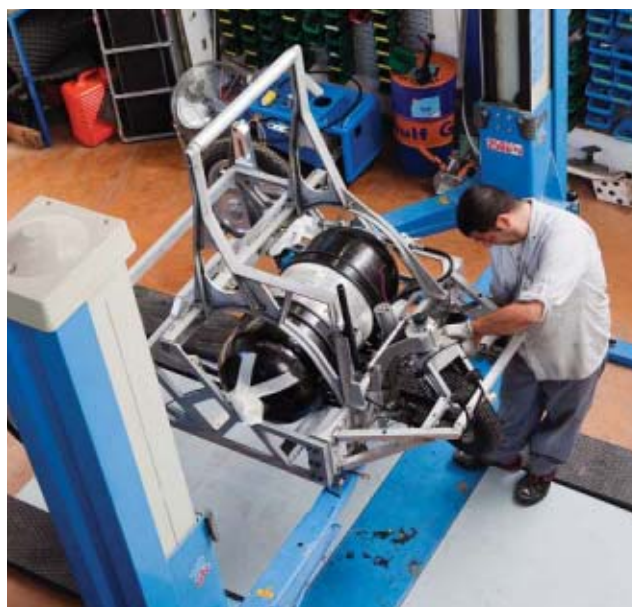
POD SQUAD: Workers at Motor Development International are busy readying AirPod prototypes at the company's fabrication facility near Nice, France. Viewed from underneath its curvaceous shell [left], the AirPod reveals an aluminum frame, which encloses a composite tank holding air compressed to 350 bars [middle]. A steering wheel would be impractical, because the driver's door is located at the front of the vehicle. The solution is a joystick placed next to the driver's right hand [right].
