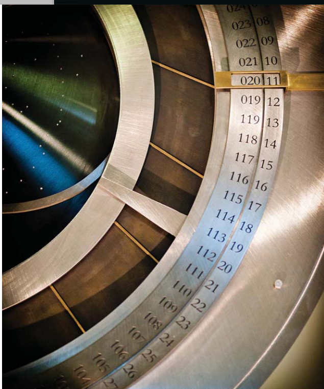
SHOW TIME: Although the clock will keep time internally, it will display only the year, and its display will update only when visitors wind the clock. PHOTO: SETH MCANESPIE
