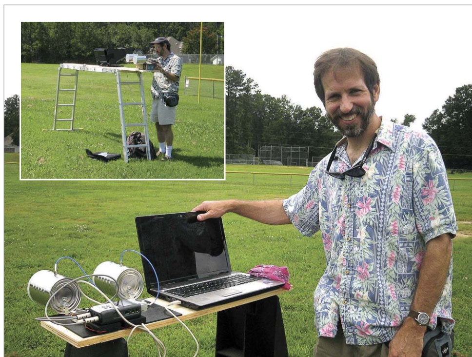
FIELD TESTS: Ranging is done in place, but for imaging the gear must be moved laterally [inset]. PHOTOS: GRACE SCHNEIDER
