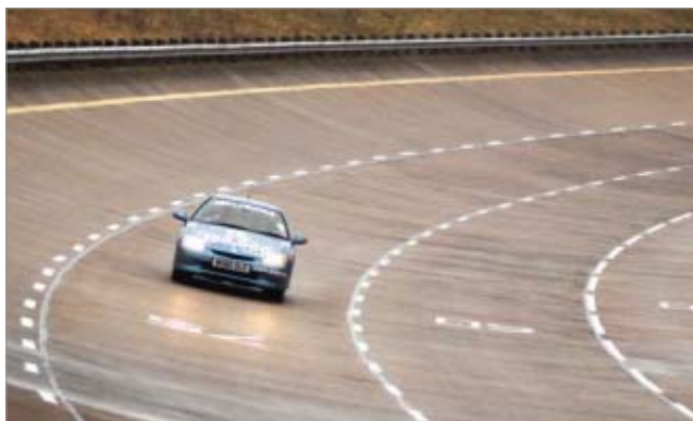
BATTERY TEST: A hybrid-electric vehicle is put through its paces using a combination ultracapacitor/lead-acid battery.
