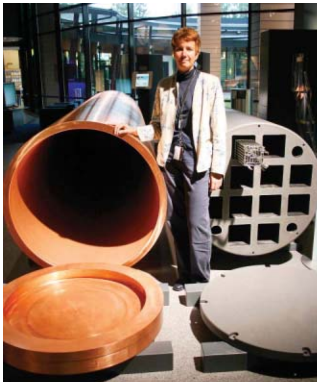
PILLARS OF FAITH: Johanna Hansen, the research and development director, stands between a 1-meter-wide copper canister and its iron interior, which Posiva says can withstand earthquakes and advancing glaciers.
