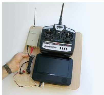
STORE-BOUGHT AND HOMEMADE: A commercial kit with brushless motors and a chassis [top] was the basis of the camera mount. A combined radio control and display screen [bottom] allows remote direction.
